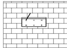
Drill holes with electric drill, make sure the holes are at least 50mm deep and 8mm wide, and then tighten the expansion tubes.
