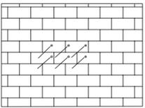
Insert the expansion tubes into the holes and tighten them. Install the bracket with the expansion screws.
